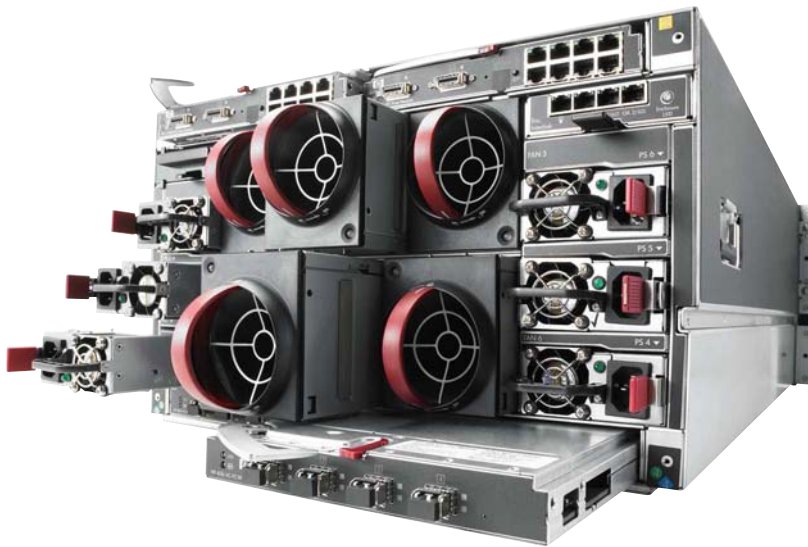
HP BladeSystem c3000 Enclosure
